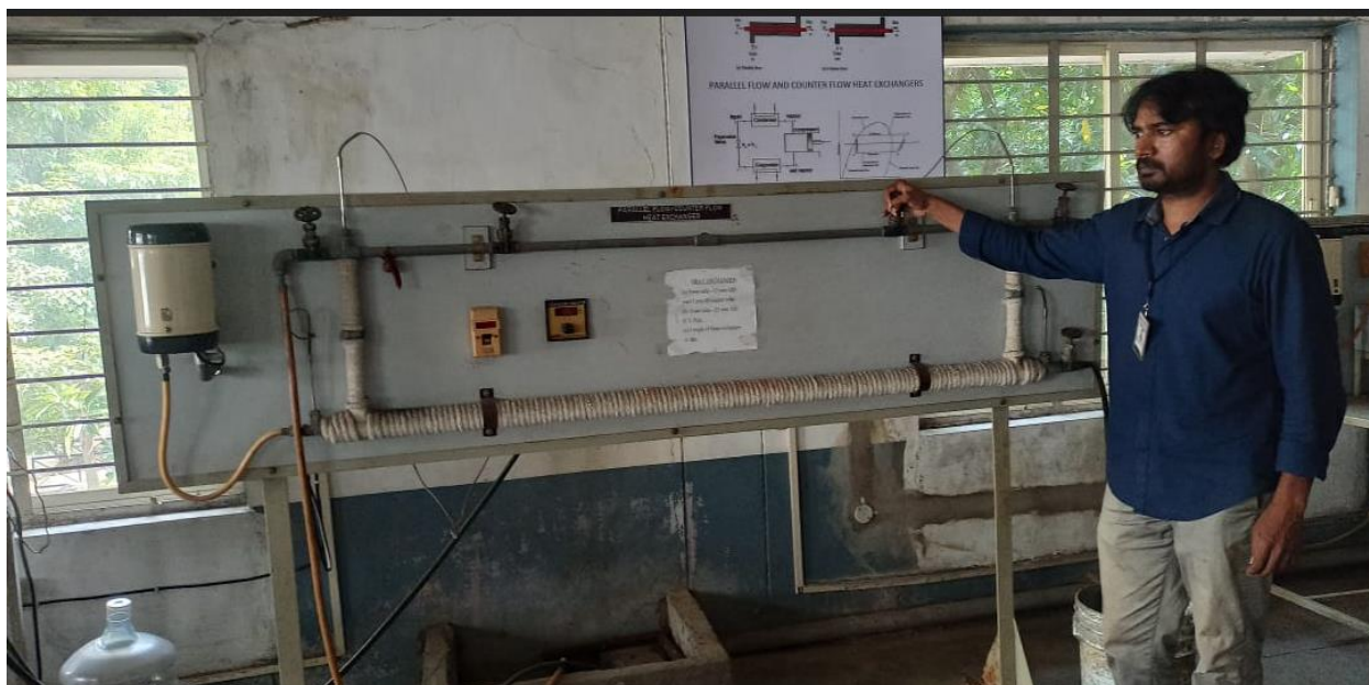
A demonstration of double pipe heat exchanger by the resource person
